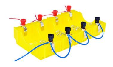
Three series with the battery case, and now the voltage of 4.5V
